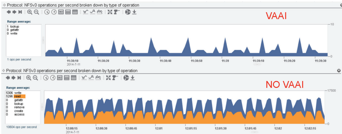
Figure 16. Oracle ZFS Storage Appliance Analytics – Offloading operation with and without VAAI for NAS plug-in enabled – NFSv3 operations per second broken down by type of operation
